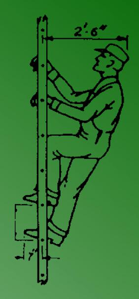
• Fixed ladders without cages or wells shall have a clear width to the nearest permanent object of at least 15 inches on each side of the centerline of the ladder.
