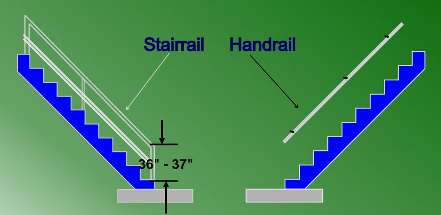
When toprail of stairrail is also the handrail it must be between 36 & 37 inches high measured from the front of the stair tread
