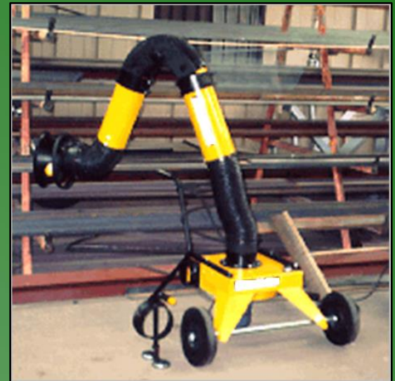
Local Exhaust Ventilation
