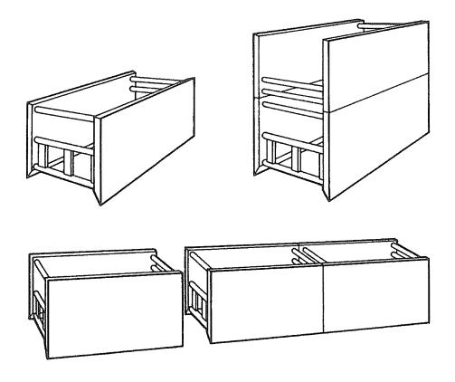
Figure 2. Trench Shields
