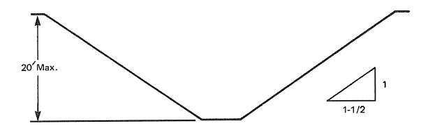
Figure 1. Excavations Made in Type C Soil
