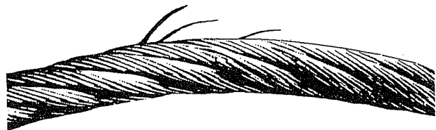
Wire Rope Fatigue Failure
