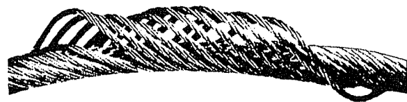
Wire Rope "Bird Cage"
