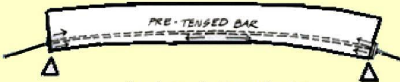
Prestressed slab - unloaded
