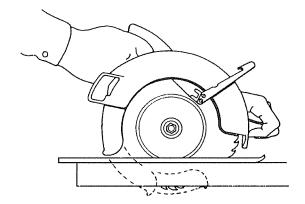
and angle grinders with wheels larger than 2 inches in diameter, disc and belt sanders, reciprocating saws, saber saws, and other similar tools. These tools also may be equipped with a lock-on control provided that turnoff can be accomplished by a single motion of the same finger or fingers that turn it on.
