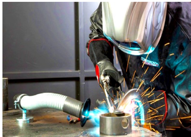
Welder using local exhaust ventilation to remove fume from breathing zone. (Photo courtesy of the Lincoln Electric Company).
