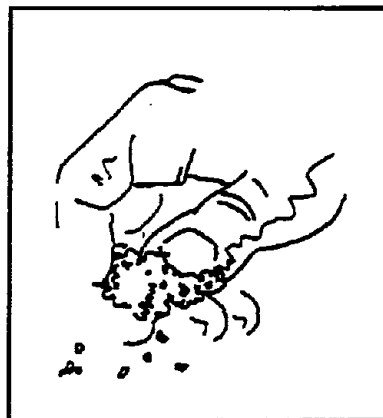
FRIABLE (CRUMBLY) ASBESTOS
